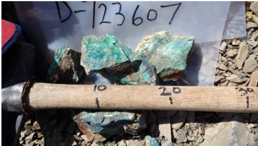
Photo 1 – Sample D-723607 – 15.55 % copper.
